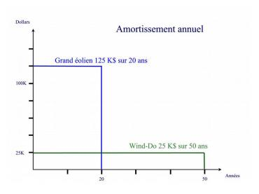
In this example, a \$2.5M giant wind turbine amortizes over 20 years cost \$125K per year for dampening. Beside that, a \$1.25M Wind-Do farm amortize over 50 years cost \$25K.
